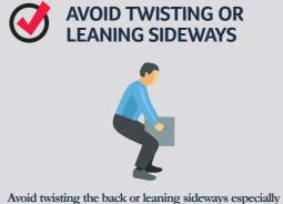
while the back is bent. Keep your shoulders level and facing in the same direction as your hips. Turning by moving your feet is better than twisting and lifting at the same time.
