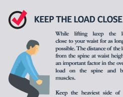
While lifting keep the load close to your waist for as long as possible. The distance of the load from the spine at waist height is an important factor in the overall load on the spine and back
